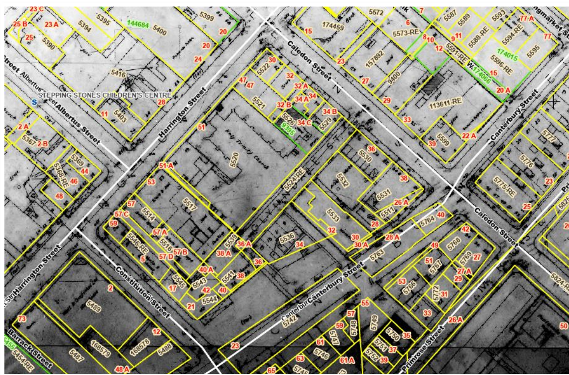
Figure 15: City Survey map (480 Series) of 1944-1966 showing building footprints with current erven and street numbers overlaid. (CoCT Map Viewer)
