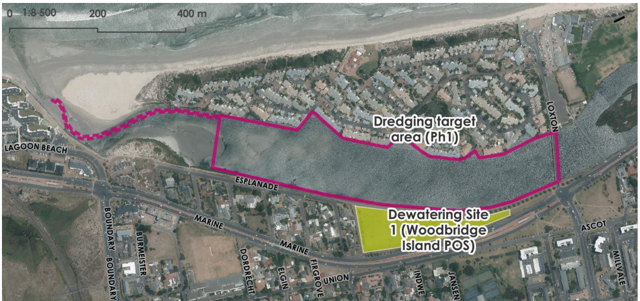
Figure 5-14: Proposed Phase 1 dredging area. The proposed first dredging action is the dredging of a canal in the mouth area (dotted line).
