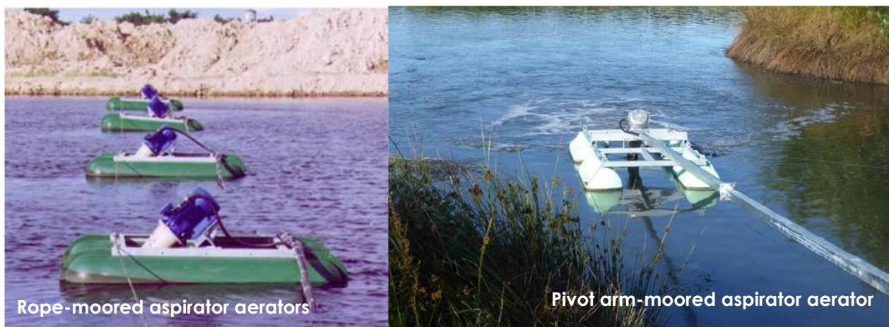
Figure 6-8: Floating aerators with mooring ropes and pivot arm
