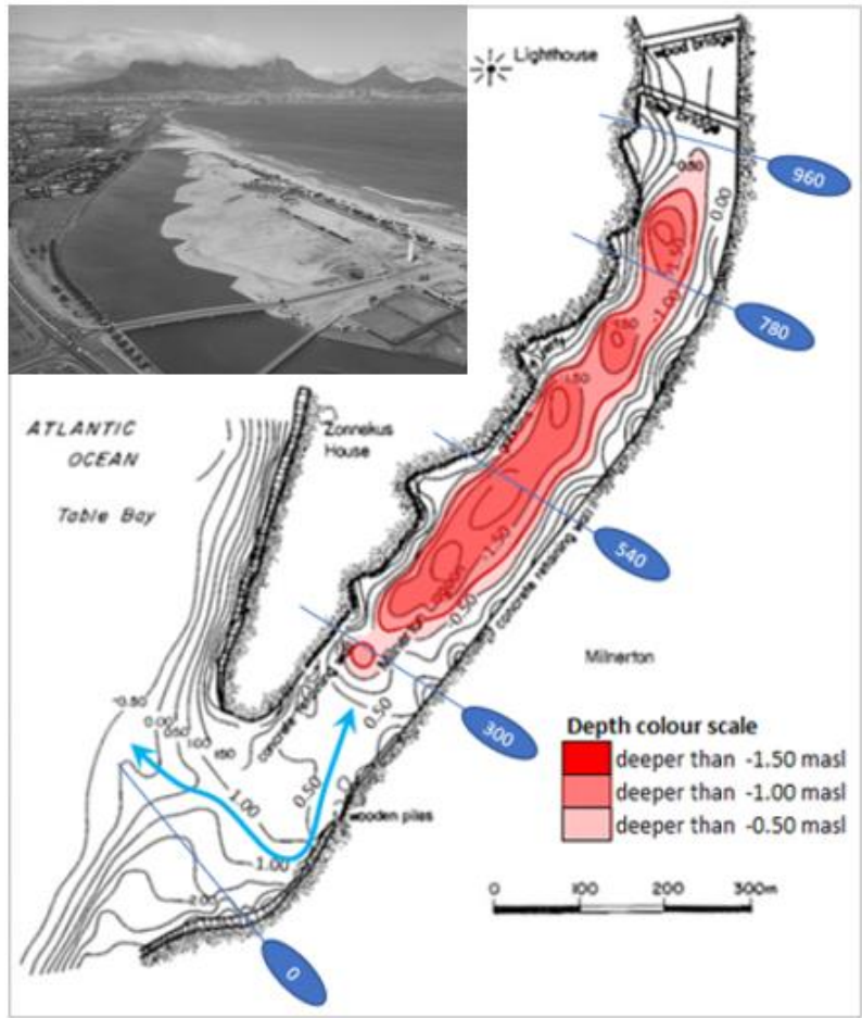
Figure 5-1. Bathymetry of Milnerton Lagoon, 26 June 1987 (CSIR, 1987) showing deeper location of dredged zones (mainly red shaded zones) during construction of Woodbridge Island Development in the 1980's (insert 1985 photograph from Independent Newspapers Archive).
