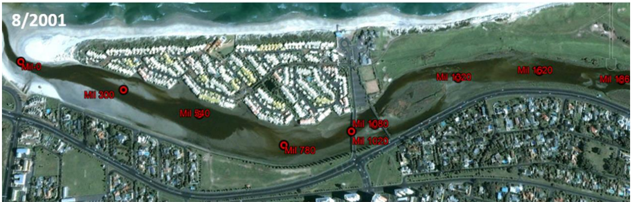
Figure 5-3: Before and after 2001 flood of about 100 m 3 /s showing scoured lower estuary and estuary mouth.
