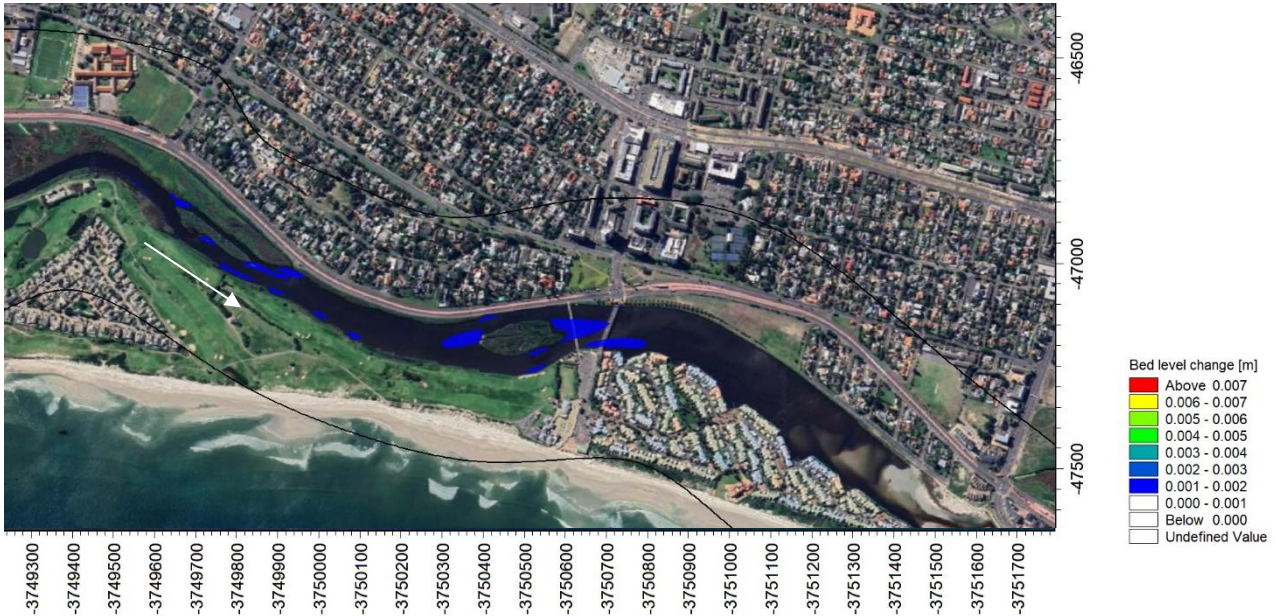
Figure 12-19. Bed level change after the Q2-flood for the Phases 1 and 2 dredged bathymetry
