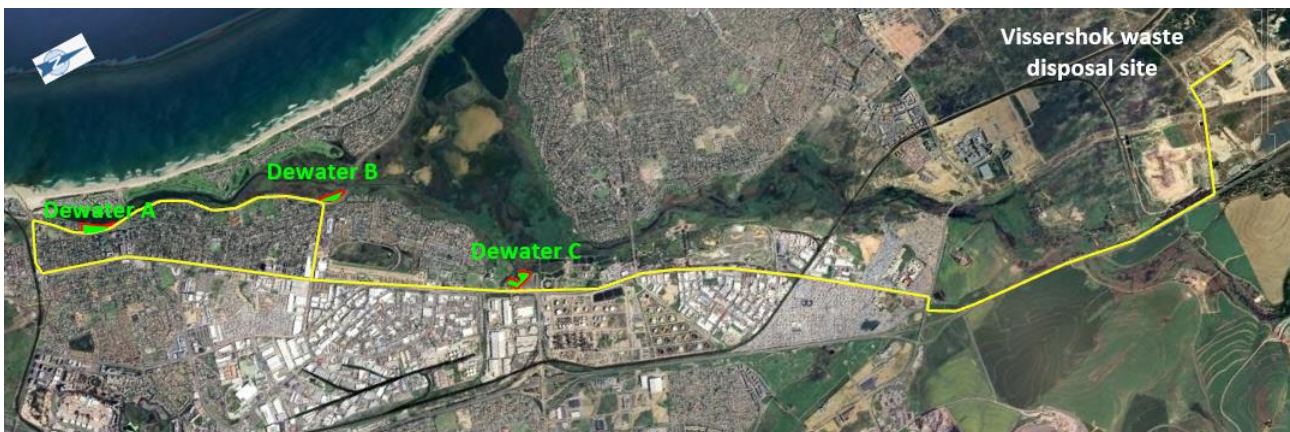
Figure 5-26: Haul route for carting dewatered material from dewatering sites 1, 2 and 3 to Vissershok waste disposal site as a provisional dredged material disposal site
