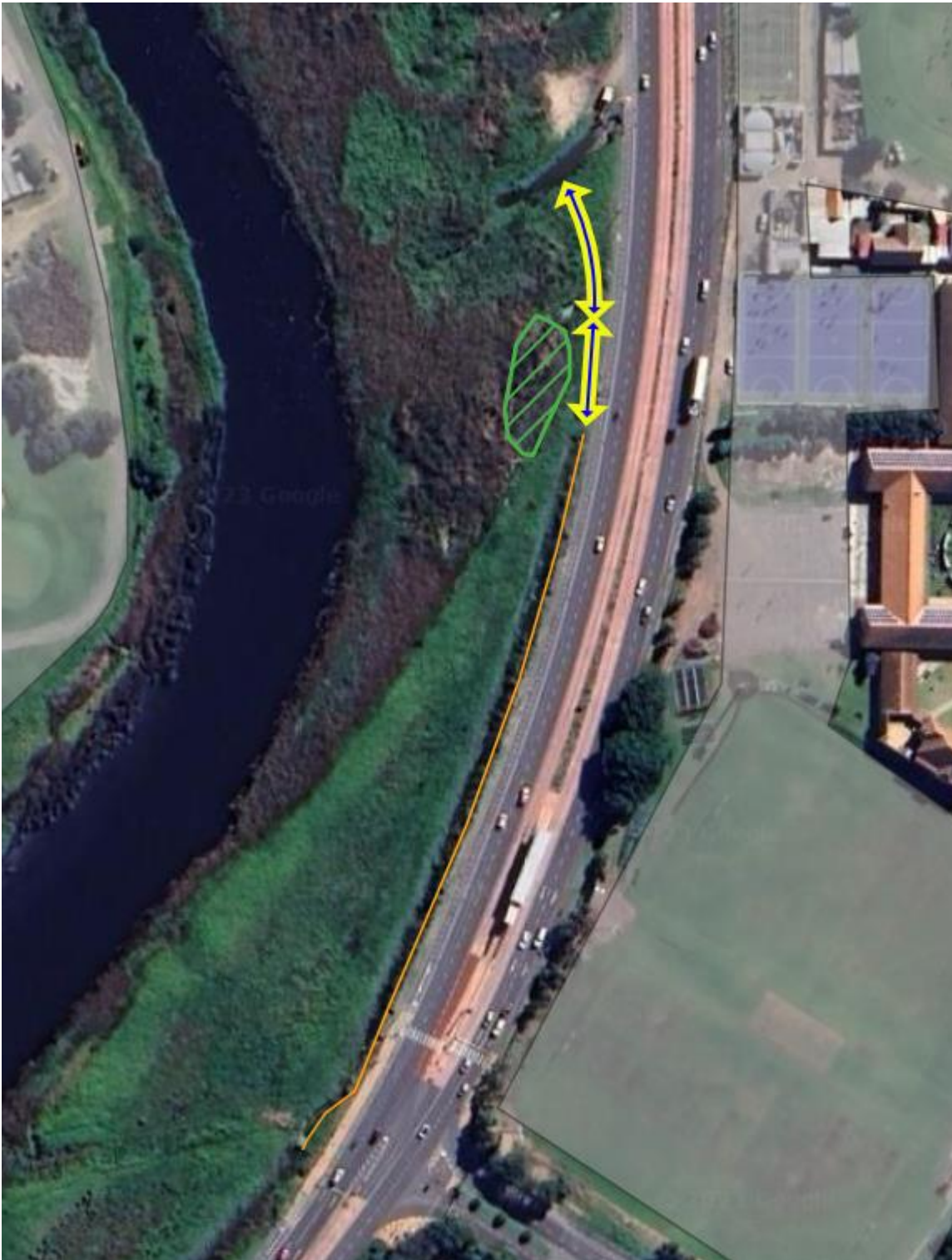
Figure 9-2. Proposed biofilter diversion channel to link with existing swale alongside Otto du Plessis Drive.
