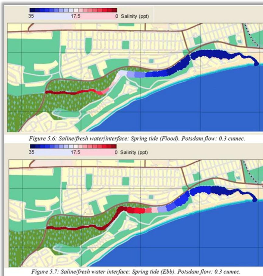
Figure 7-1. Excerpt from Botes et al (2004) showing salinity penetration in the lagoon during spring tide
