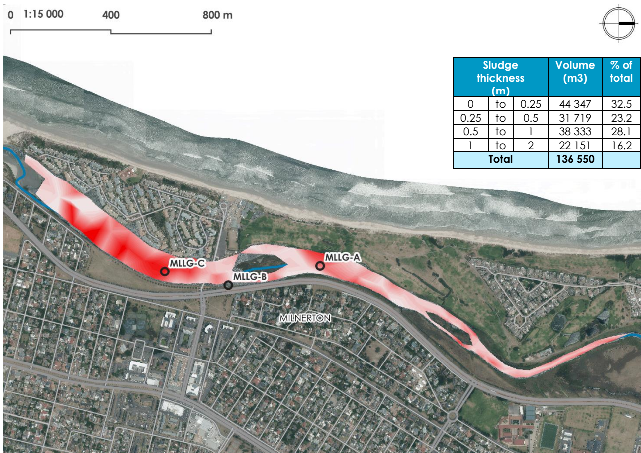
Figure 5-12: Tritan Survey's derived sludge isopach contours of sludge thicknesses and estimated nett sludge volumes per thickness ranges. Sample locations for the additional samples shown in Figure 5-11 are indicated.
