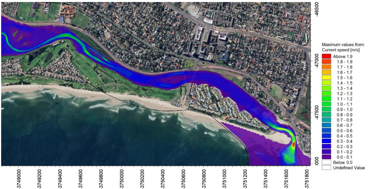
Figure 12-20. Simulated maximum flow velocities for the Q2 year flood event for the dredged scenario
