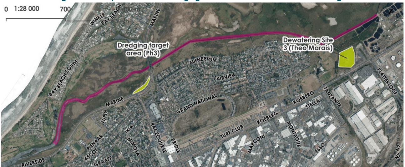
Figure 5-16: Proposed Phase 3a dredging for the removal of contaminated sludge.
