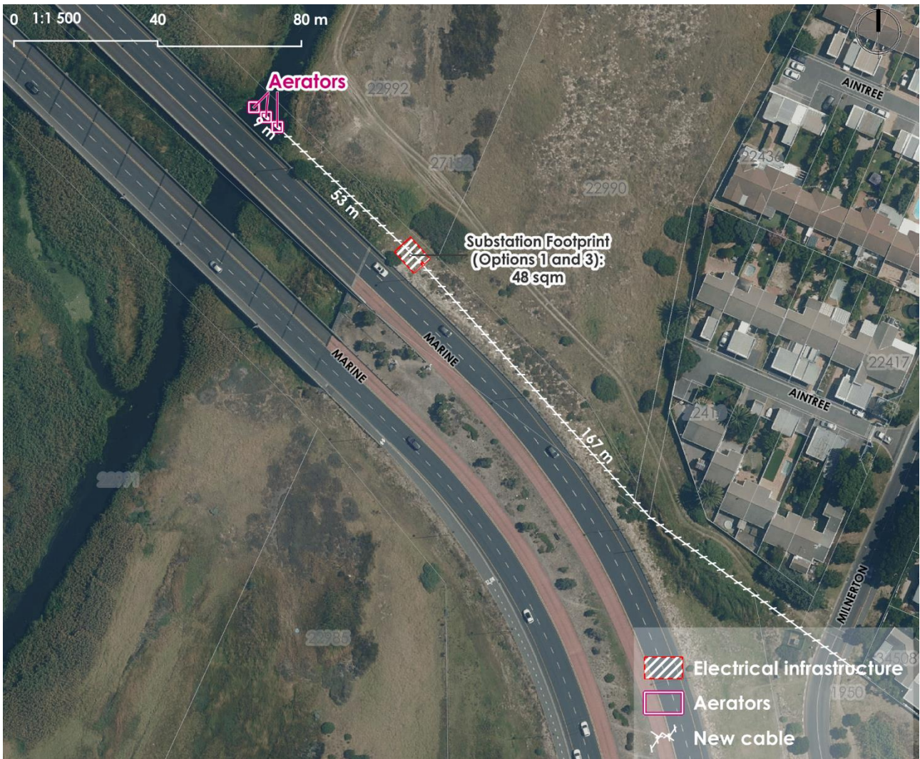
Figure 6-13. Electrical supply infrastructure routing (Upstream site)
