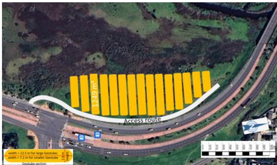
Figure 5-24: Geotextile tube dewatering site for dredging the lower part of Phase 3. Total volume of this layout, is approximately 16 800 m 3 .
