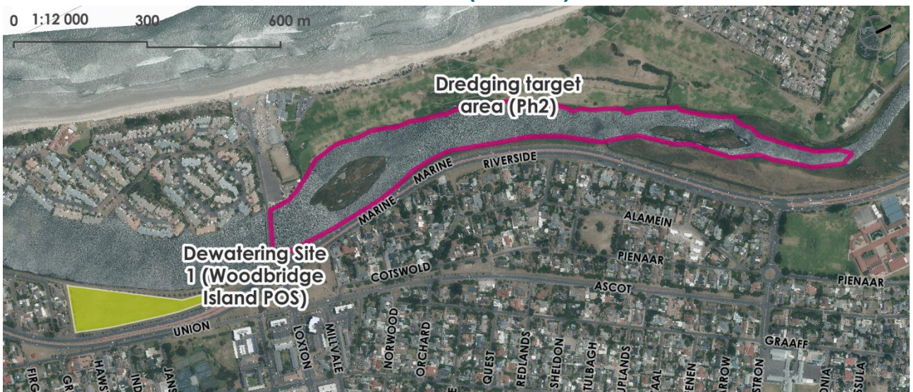
Figure 5-15: Proposed Phase 2 dredging for the removal of contaminated sludge.
