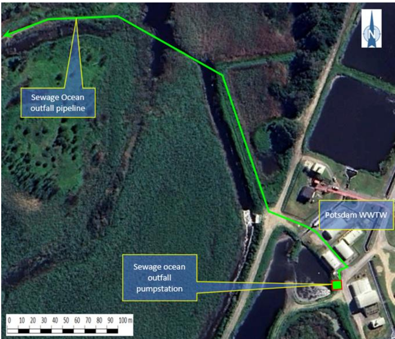
Figure 8-2. Location of ocean outfall pumpstation inside the Potsdam WWTW
