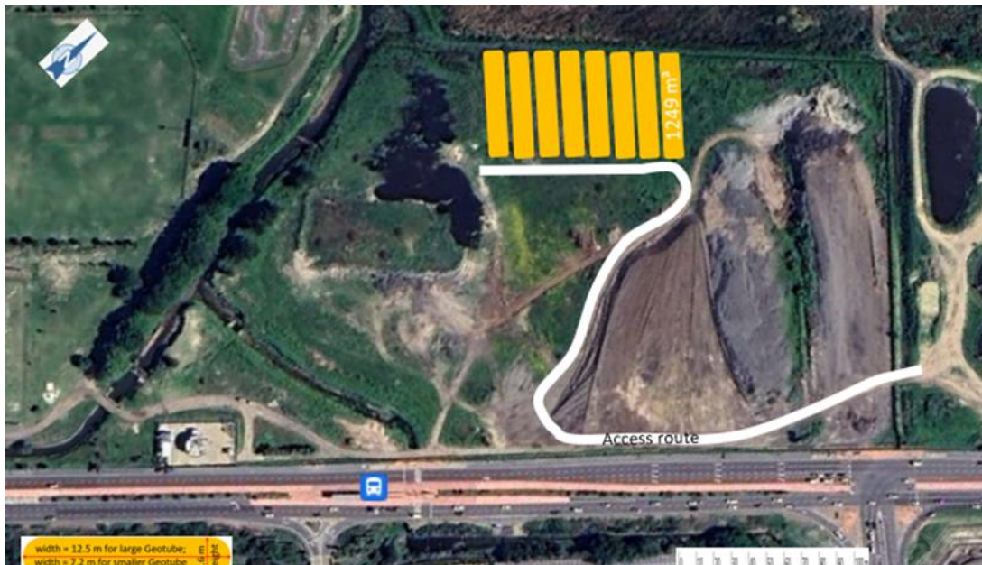
Figure 5-25. Geotextile tube dewatering site for dredging Phase 3. Total volume of the layout shown, is approximately 10 000 m 3 for each of the two branches shown which is much more than required for Phase 3.
