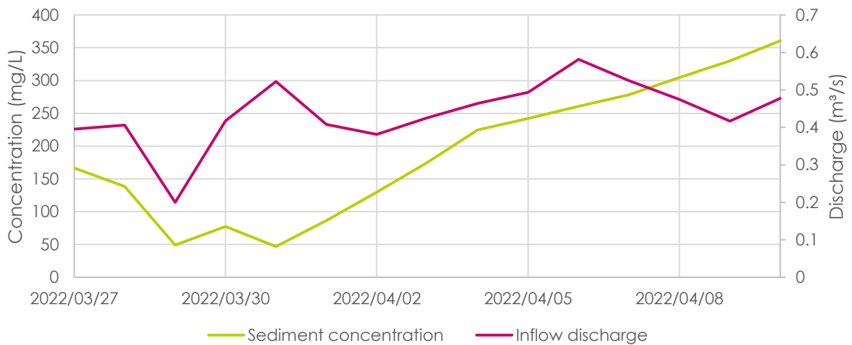
Figure 12-8. Sediment inflow concentration and inflow discharge for the two-week spring tide period
