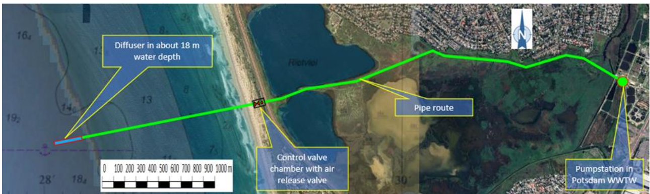
Figure 8-1. Possible layout of a marine outfall for discharging Potsdam WWTW effluent in the ocean indicating the locations of the pipe route pump station in Potsdam WWTW and diffuser in the ocean are shown.
