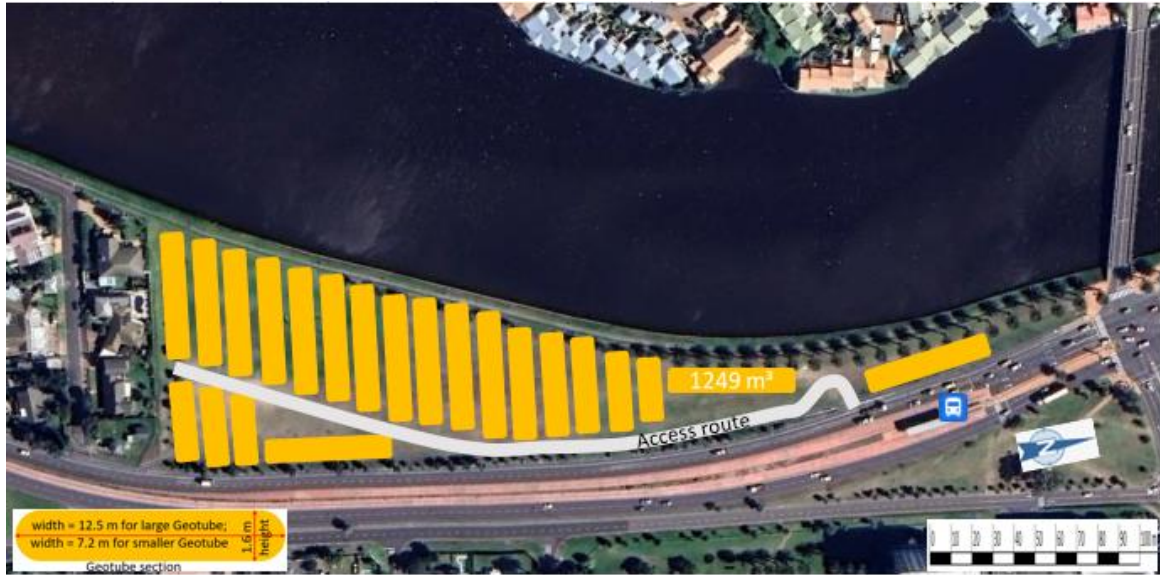
Figure 5-23: Geotextile tube dewatering site for dredging Phases 1 & 2. Total volume of this layout shown, is approximately 22 000 m 3 .
