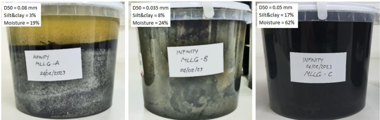
Figure 5-11: Additional samples of sludge material taken on the south side (A), between (B) and on the north side (C) of the Woodbridge Island bridges
